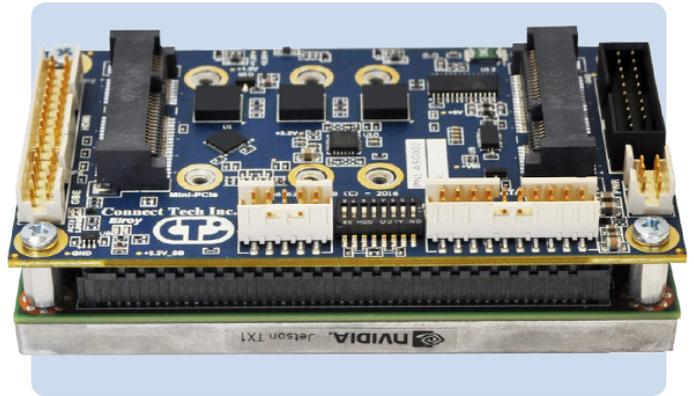
Connect Tech's new Elroy Carrier for Jetson TX1 is designed with rugged use in mind and harkens true to the adage that great things come in small packages. Even at just 87mm x 50mm, it still exposes many of Astro and Jetson TX1's great features and peripherals.
