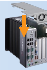
3. Replace it by plugging the hot-pluggable fan module cover into the fan connector on CPU board
