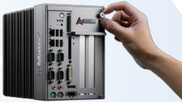
1. Undo the thumbscrew by hand
