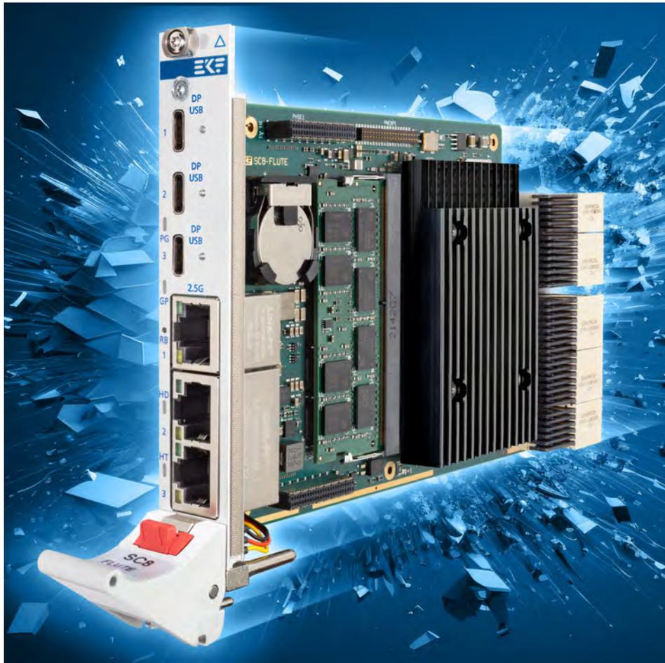
SC8-FLUTE - SODIMM on Top of Soldered RAM
