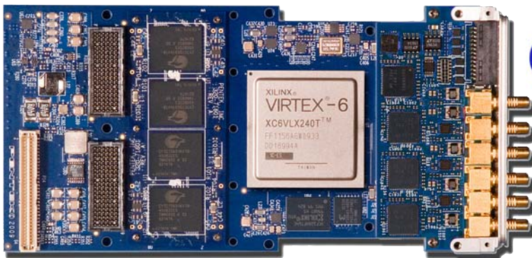
Pentek XMC Software Radio Board with Virtex-6 FPGA
