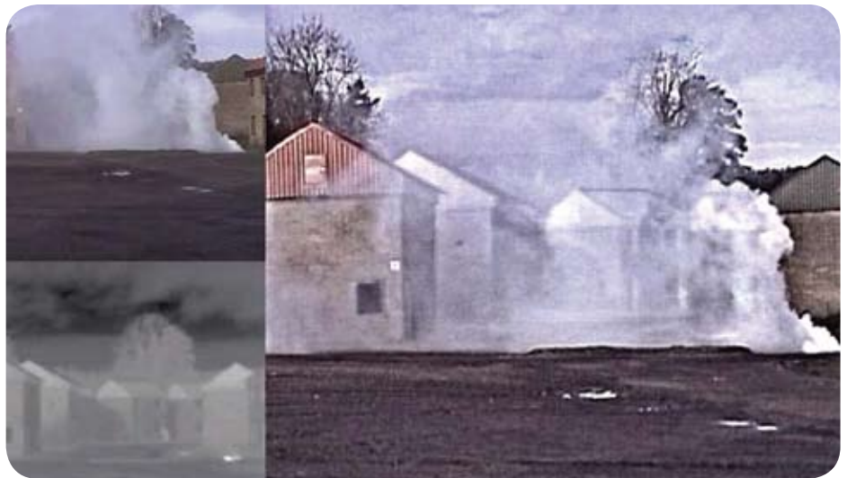
Image fusion combines multiple sensor inputs into a single, superior image.
